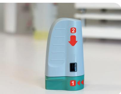
**ZENEO® is a prefilled, single-use device capable of propelling a medical formulation through the skin in only 50 milliseconds.** Its injection parameters are entirely factory-set according to the viscosity, dosage and injection route (subcutaneous or intramuscular) of the drug formulation. For a needle-free auto-injector, this versatility is unmatched anywhere in the world.
